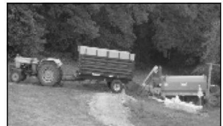
The nuts are tipped into the washer, which separates the shells from the husks
