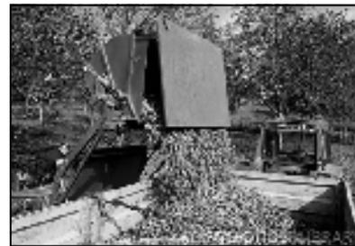
Tractors equipped with giant claws grip each tree and literally shakes the nuts off the branches, the nuts falling in a massive shower onto the newly cleared ground. These are in turn swept up into huge
