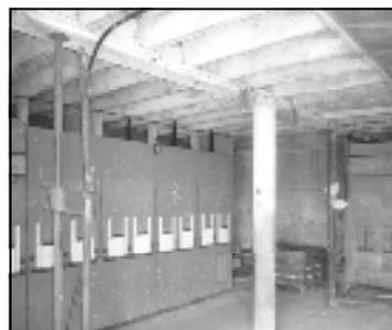
The washed nuts are tipped out of tractor trailers from the floor above, into huge drying hoppers.
